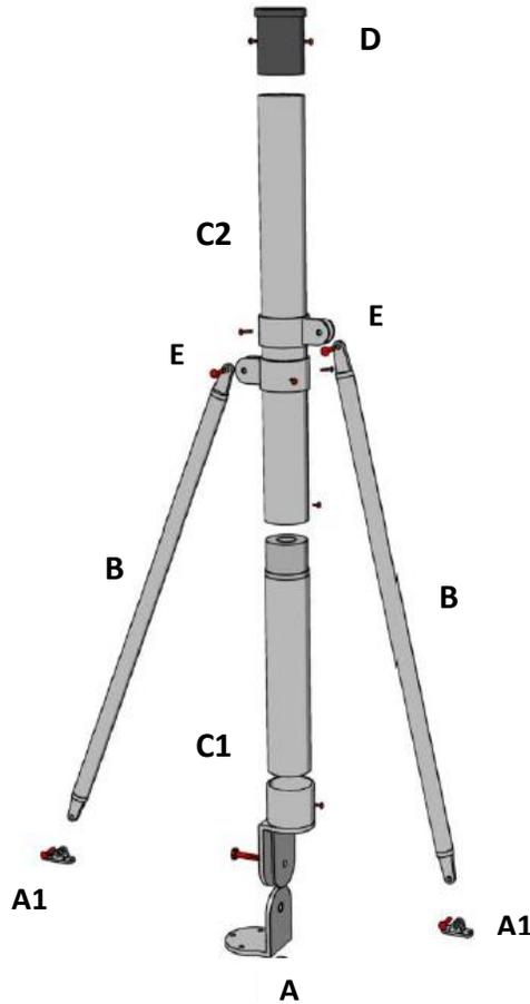
Mast components made of polished 316L Stainless Steel.
