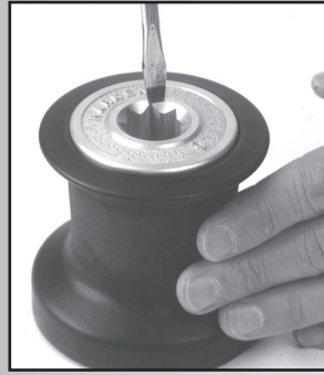
Use screwdriver to open winch
