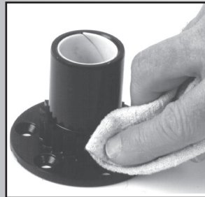
Clean all parts with solvent.
