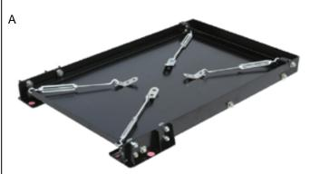
strong low profile steel slide that extends out 80% allowing access to your Engel freezer in confined spaces. Turn buckles and tabs (included) attach your freezer securely to the slide. Sealed roller bearings prevent jamming due to sand or dirt. Safety latch - locks tray for safe storage. Tough enough for off-road vehicles. Slide can also be used for generators.
