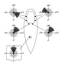
Be also aware that selftailing arm is positioned correctly. We recommend to have the selftailing arm positioned within the shaded area. On 12ST and 28ST the position of the selftailing arm is fixed, making it very important to establish the proper location of the holes prior to drilling these in the deck. On all other models, the selftailing arm can be placed in several different positions after having installed the winch.
