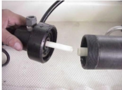
Remove the opposite end cap and install the Z-Brane ground end cap.
