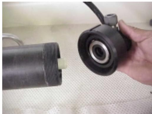
The cable assemblies should be complete as supplied. If you need to modify the ground wire or the power cable, use heat shrink to seal the terminations. **DO NOT** modify the high voltage cables. Make sure that they are clear from moving items that could cause abrasion on the cable.
