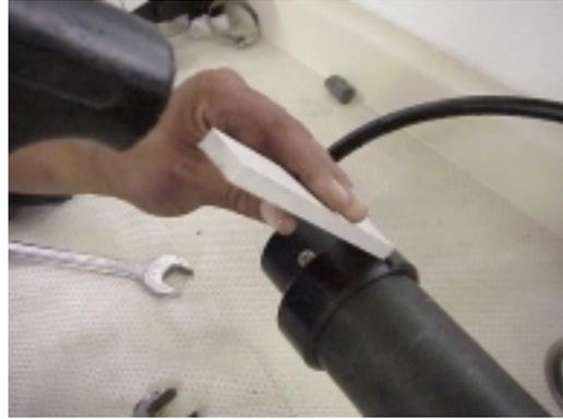
Gently pry out the end cap while you are unscrewing the retainer ring.
