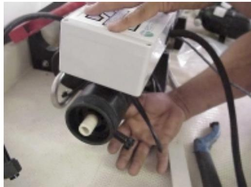
Route the power cable to a fused power source. The Red wire is the positive feed (+). The black is ground (-). Fuse the power lead with a 5A fuse.
