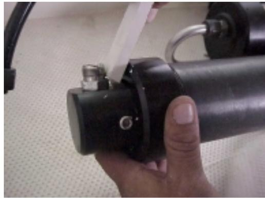
Put a bit of silicone grease on the pressure vessel threads. Line up the Z-Rod with the product tube and install the new end cap. Do not force the rod into the tube.
