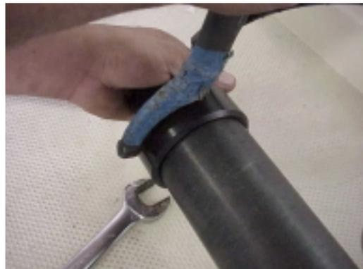
If the ring removal tool is not available a block of wood and a mallet will work as well.
